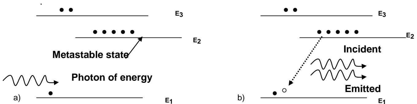
Figure 6 – Emission of photons from the metastable state.
